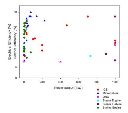
Figure 17. Electrical efficiencies of biomass conversion technologies based on power output [58].
