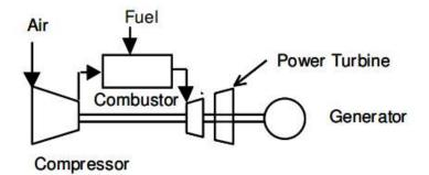
Figure 65: Components of simple-cycle gas turbine [28]
