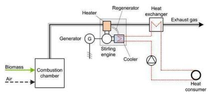
Figure 69: System diagram for a biomass CHP unit with a stirling engine [32]
