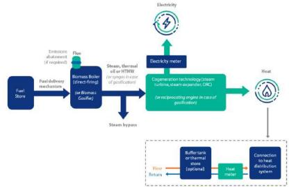
Figure 12: Typical biomass CHP components [38].
