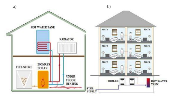
Figure 1. Scheme of direct heating system: a) single-family house [3], b) residential block [4].
