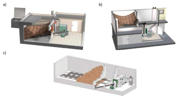
Figure 40. Examples of storage and loading solutions for chips [27]: a) chips store and the boiler room are on the same level (leaf reel and 2 feeders); b) chips storage and boiler at different levels: horizontal leaf reel, feeder, slope system; c) hydraulic floor systems.
