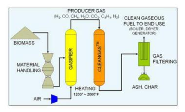
Figure 15: Example of two-stage gasification [44].
