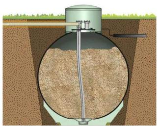
Figure 34. Underground pellet storage silo [16].
