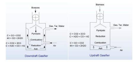
Figure 60: Fixed-bed gasification systems [17]
