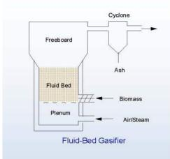
Figure 61: Fluidized-bed gasification systems [17]
