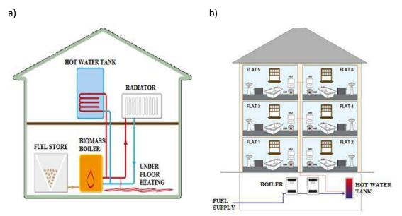
Figure 25. Scheme of direct heating system:
