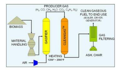
Figure 59: Example of two-stage gasification [16]
