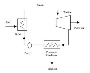
Figure 64: Steam turbine CHP system [27]
