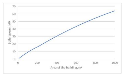
Figure 44. Thermal power of the boiler vs. Heated surface area of the building (in a temperate climate)<sup>8</sup>.
