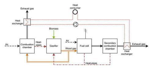
Figure 68: System diagram for a biomass CHP unit with fuel cell [29]
