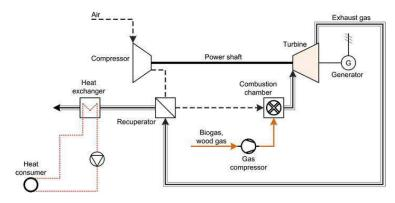
Figure 66: Microturbine-Based CHP System [30]
