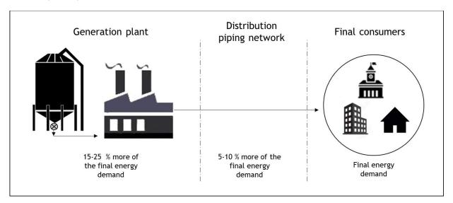
Figure 48. Basic scheme of the energy to be supplied in each part of the district heating system.
