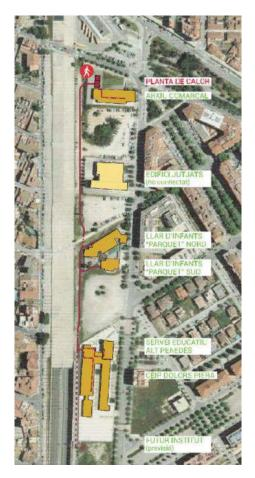
Figure 51: Scheme of the District Heating in Vilafranca del Penedés.
