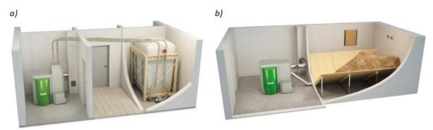
Figure 36. Examples of connecting a pellet boiler with a storage system [19].
