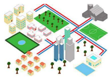
Figure 47. Scheme of a District Heating [2].
