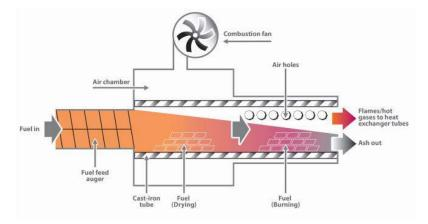
Figure 57: Fixed grate boiler [13]
