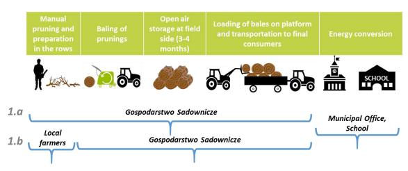
Figure 6. The logistics value chain of biomass utilization for energy purposes in rural area [29].
