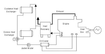
Figure 67: Closed-Loop Heat Recovery System for a Reciprocating IC Engine [27]
