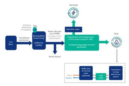
Figure 53: Typical biomass CHP components [1]
