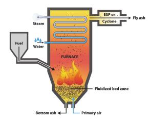
Figure 58: Fluidized bed boiler [14]
