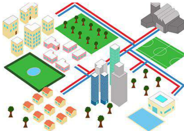
Figure 8. Scheme of a District Heating [32].
