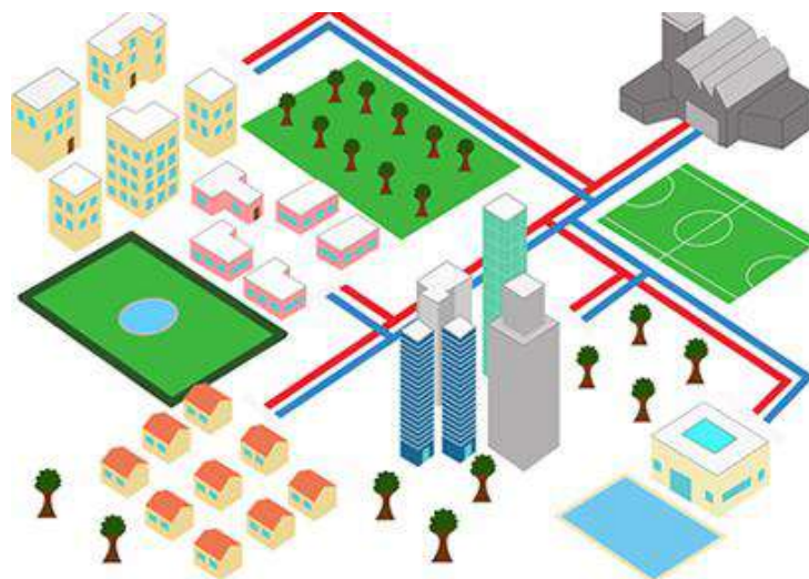
Figure 1. Scheme of a District Heating [2].
