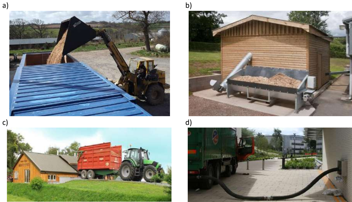
Figure 14. Chips deliver options, depending on storage scenarios [24]: a) tipped delivery into a bulk fuel store with tele handler chips moving; b) fast feed auger delivery; c) ramped delivery; d) blown delivery.
