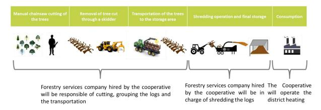
Figure 1 Diagram of value chain operations (forest residues)
