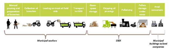
Figure 34 Diagram of value chain operations (urban prunings)
