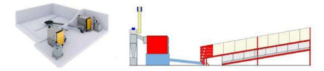
Figure 5 Example of feeding system and biomass boiler for the forestry biomass (left) and herbaceous biomass (right).
