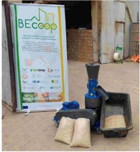
Drive type: Electric Capacity: up to 100 kg/h Motor power: 4 kW Voltage: 400 V (3-phase power supply) Engine speed: 1500 rpm Die rotation speed: 250 rpm The diameter of the holes in the die: 6 mm Die thickness: 32 mm Die diameter: 150 mm Number of rollers: 2 pcs. Number of knives: 1 pc. Length: 900 mm Width: 500 mm Height: 1100 mm Weight: 180 kg
