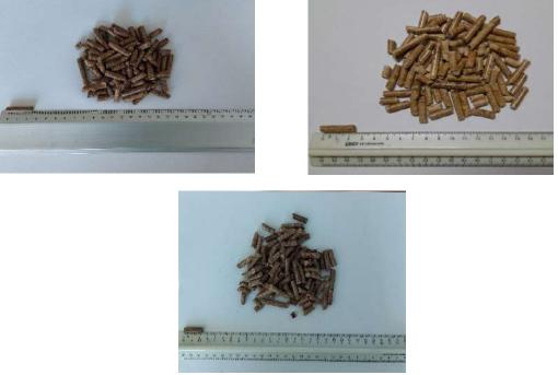
Figure 27. Top left; Wood pellets. Top right; urban waste wood with coffee grounds (CU10). Bottom; sawmill residues with coffee grounds (CS10).
