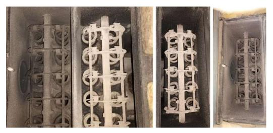
*Figure 5. Images of the heat exchanger of the biomass boiler after the test.*
