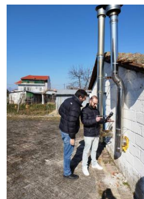
Figure 39. Boiler installation and flue gas emissions monitoring.
