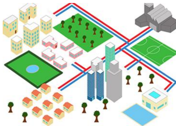
Figure 32. Scheme of a District Heating system
